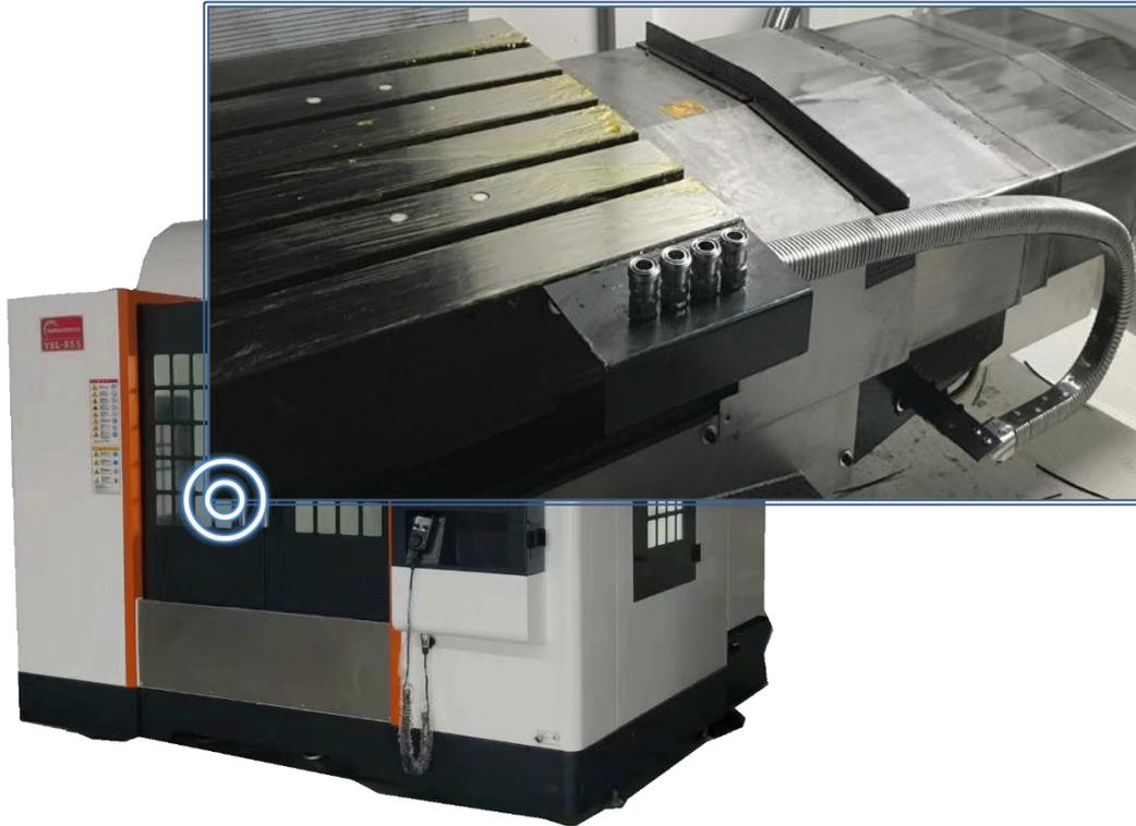
≡ Help users to pre-install pneumatic fixture pneumatic interface configuration on the workbench, convenient for users to connect pneumatic fixture. Small tools holder hole greatly reflects great sincerity.
