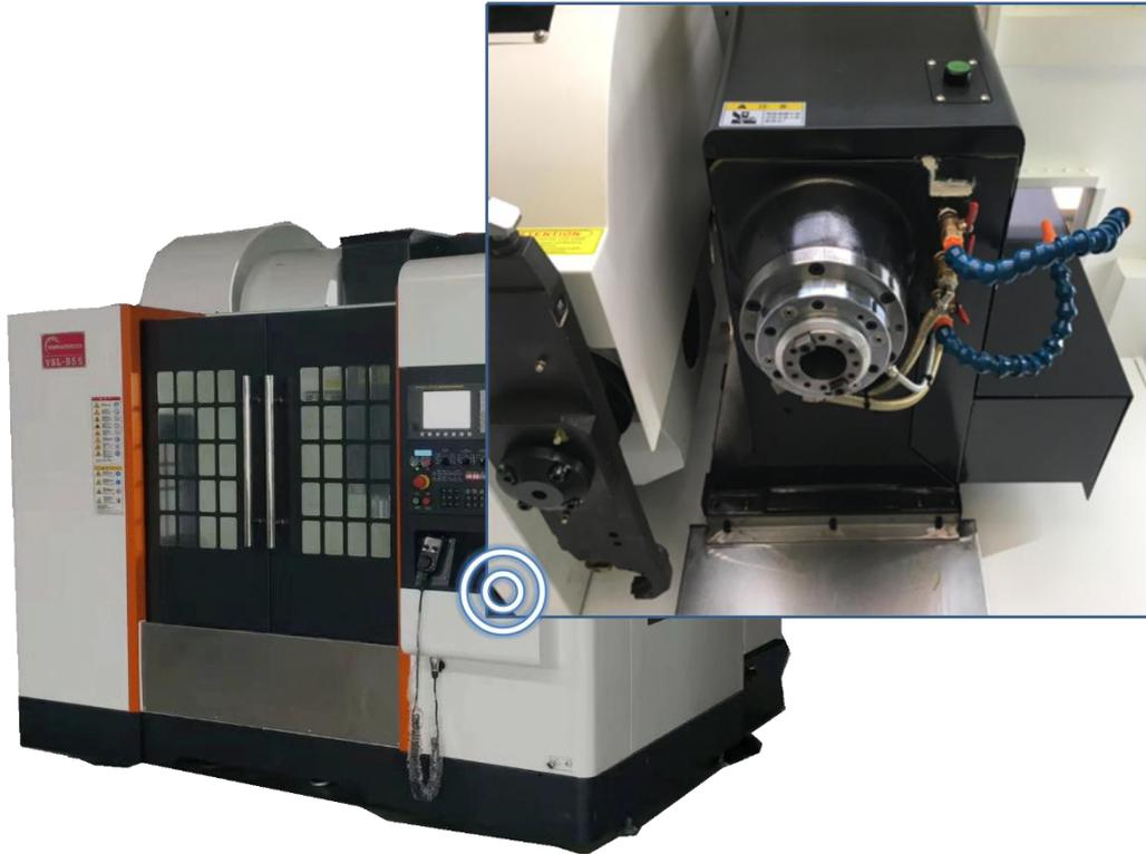
≡ The unique protection function of the spindle "air curtain" in the processing process, the spindle cone hole will eject "air curtain", effectively prevent the water and gasoline mist in the processing process, dust particles into the spindle cone hole, to a great extent, to protect the spindle, prolong the service life of the spindle, enhance the processing stability, accuracy, and greatly reduce the failure rate.
