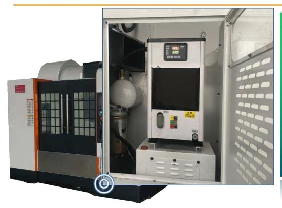
**■** Unique spindle constant temperature oil cooling technology fully automatic oil spray cooling function all-weather spindle working temperature and set temperature real-time monitoring and comparison, adjust when the spindle working temperature reaches the limit temperature, the automatic oil cooling system starts to work, timely cooling to ensure the spindle working performance, prolong service life, enhance work efficiency.
