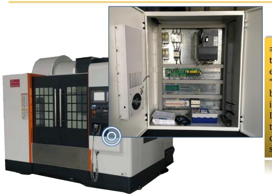
■ User's processing safety is always put in the first place by Yongshuo. Yongshuo's electrical system is equipped with a unique "phase-out" and "virtual" protection system, but in the installation of wiring, if the voltage is unstable, or there is "phase" or "virtual" or" If the phenomenon of "phase absence" occurs, the system will trip automatically to prevent damage to the control board and circuit system caused by over voltage or current.
