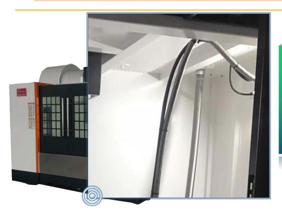
≡ Yongshuo Standard Configuration has built-in four-axis and five-axis electrical interfaces for users by default. Even if users do not need it now, when upgrading is needed, they only need to buy a turntable, plug-and-play, without more disassembly and installation, which greatly facilitates users.
