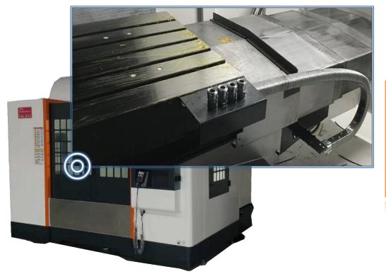
≡ Help users to pre-install pneumatic fixture pneumatic interface configuration on the workbench, convenient for users to connect pneumatic fixture. Small tools hoder hole greatly reflects great sincerity.
